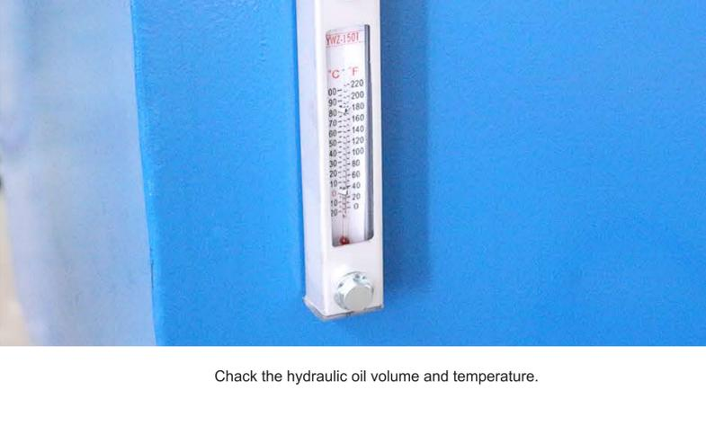
Check the hydraulic oil volume and temperature.
